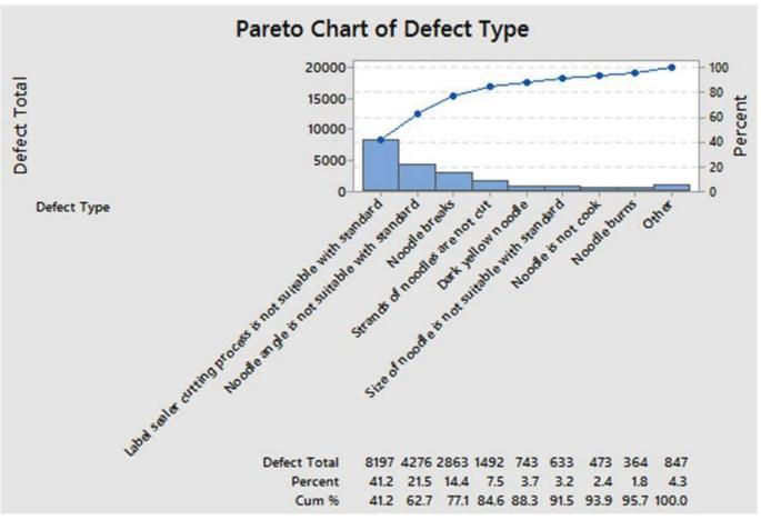
Figure 3: Pareto Diagram Number of Defective Products
